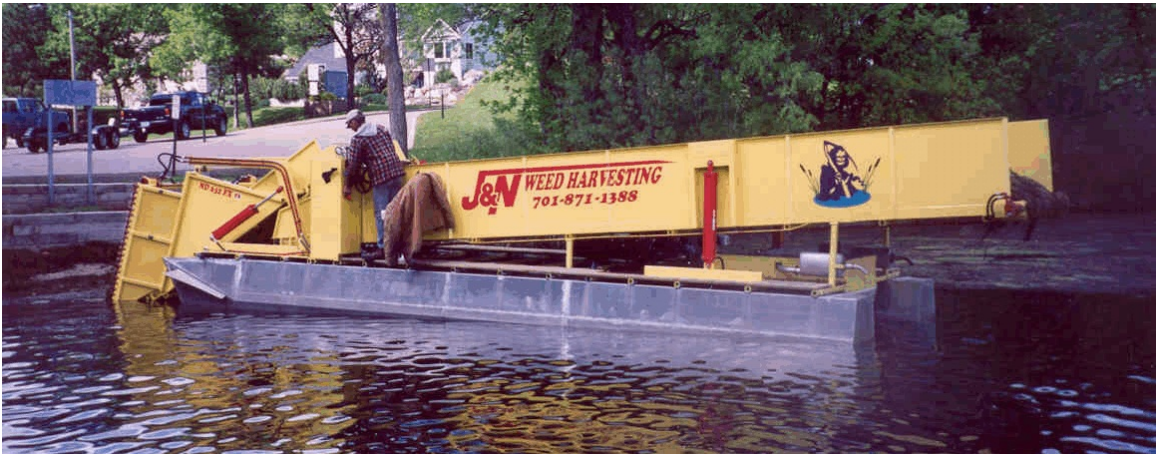
Figure 30. A mechanical harvester is recommended for picking up fern pondweed in the shallow southwest bay if plant management is considered.
