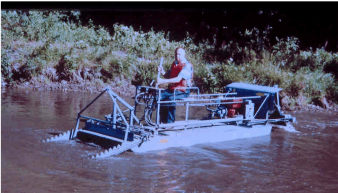
Figure 31. Hockney-type weed cutter or a mechanical harvester could be used to cut one or two channels through the cabbage on the west side of VanVliet Lake.
